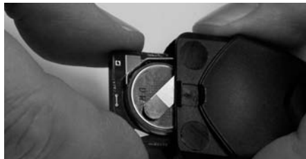
4 With the spacer removed, gently tap on a solid surface to remove the PCB unit,
